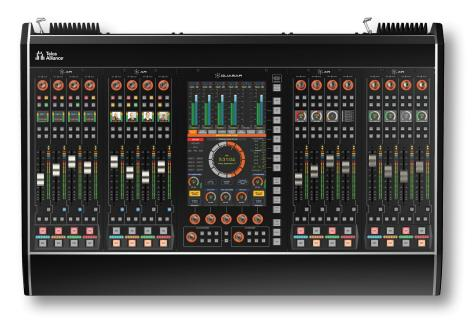
Quasar XR is our top-of-the-line mixer featuring extensive metering built into the surface right where it needs to be—on every channel display and next to each fader, as well as on the monitor module. These LED meters allow users to live mix rather than merely confidence monitor, giving users active control over their environments for the best possible outcome.
